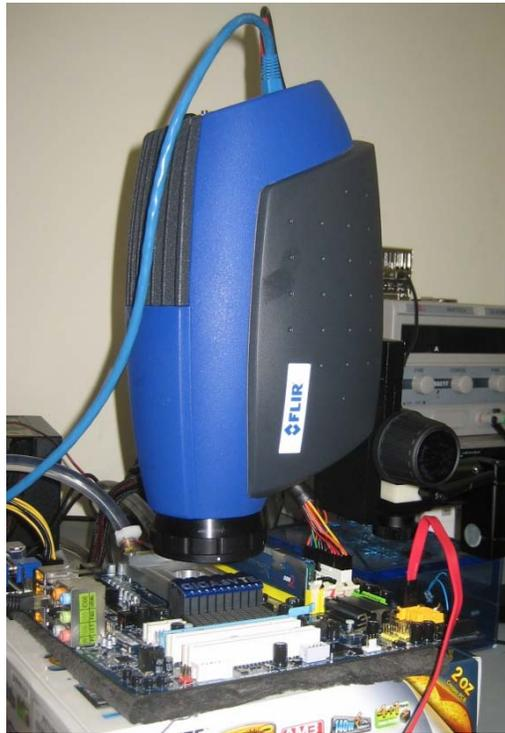
*Figure 16: Image of IR Camera and Motherboard*
