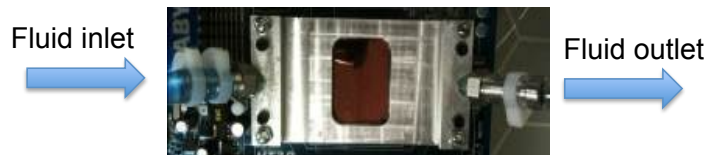
Figure 2.5: Infrared-transparent oil-based heat removal system.
