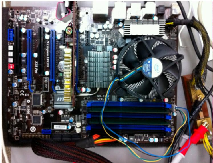
Figure 4: Motherboard used for experimental data, containing an Intel i7 processor.
